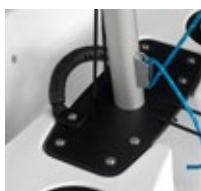
Extra strong Mast thwart mounted with 8 stainless steel crews.
